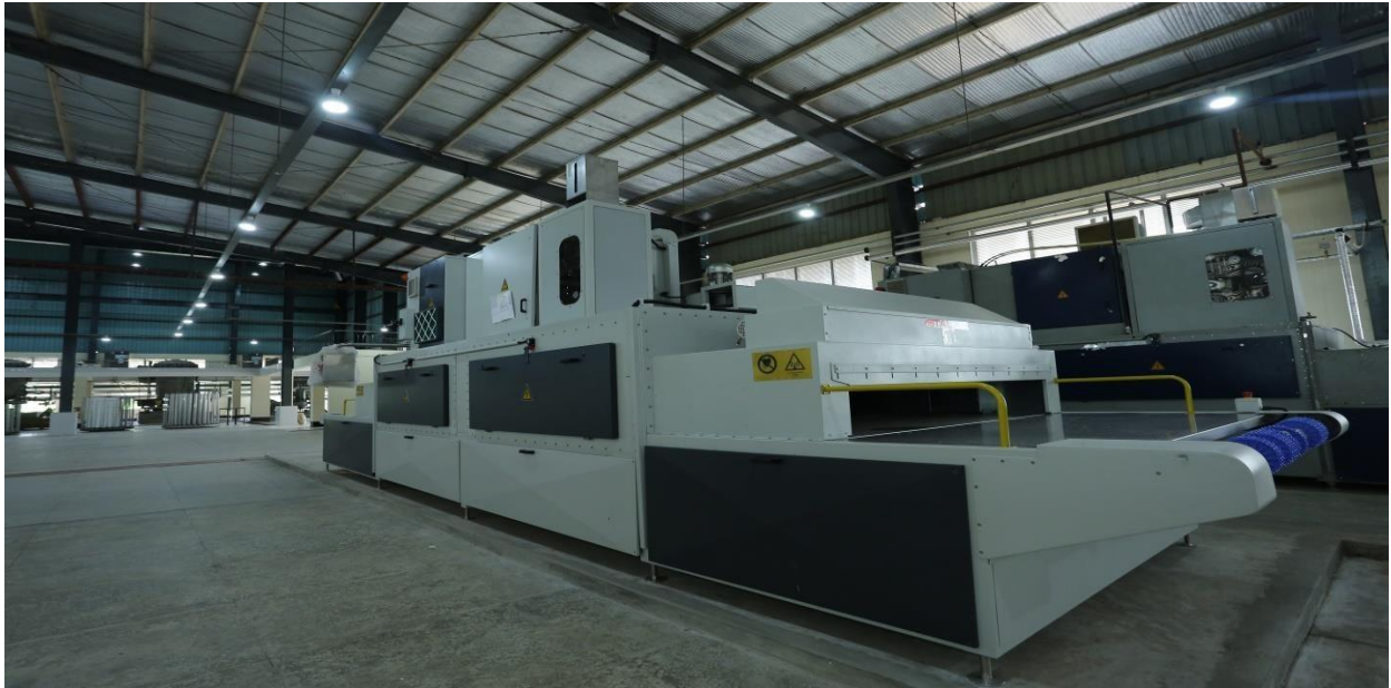
Figure: A pictorial representation of RF Dryer
