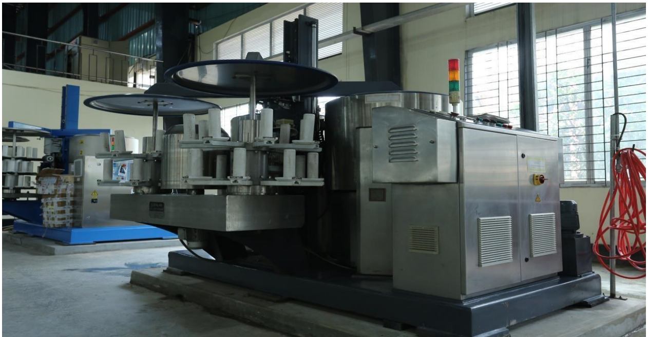
Figure: A pictorial representation of Hydro Extractor
